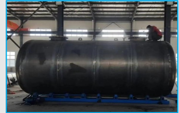
Pressure vessel and Tank Fabrication
